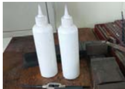
Unlabeled hazardous chemicals
